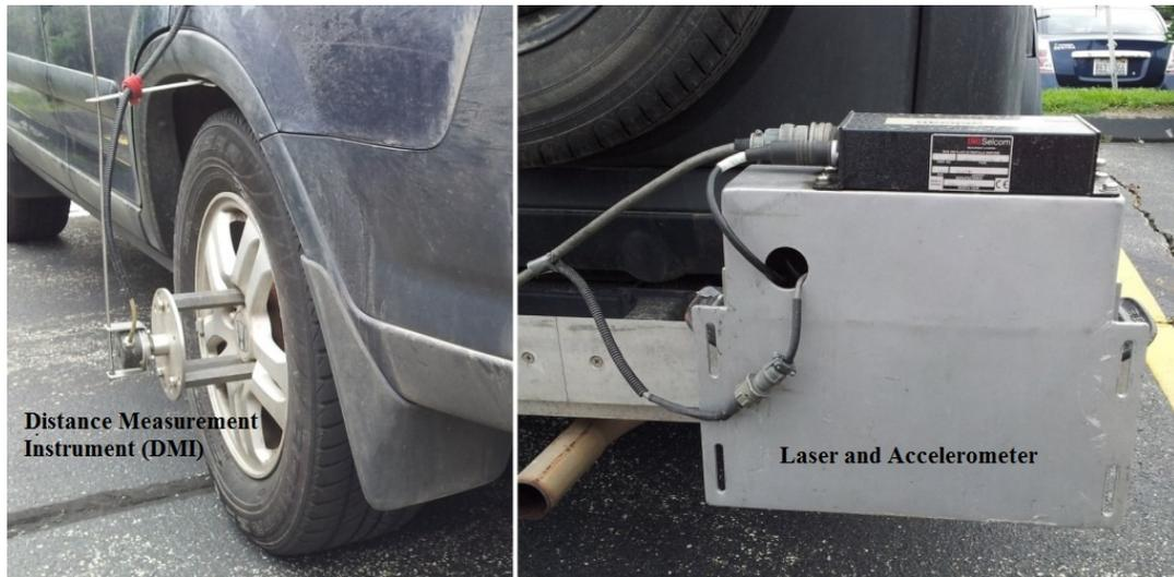
Figure 2.2 Automated pavement profiler and equipment on a typical data collection van
