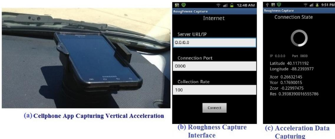
Figure 3.1 Illustration of smartphone based roughness capture system
